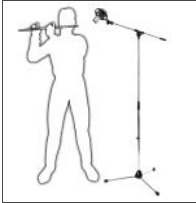
Fig. 8: Miking the flute with a single microphone.
